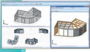
Klaes 3D provides the proper solution for all materials: aluminum, timber, timber-aluminum as well as PVC systems can be combined individually. Klaes 3D is based on a highly flexible and open data concept that integrates individual solutions and custom construction methods. You can store your own profile systems and construction details or use existing master data packages and adjust them to your individual requirements.
